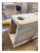
**Step 8:** Set back on. Align the back's top edge with the 1-piece side and screw in place. As with the front, (2) screws go into the bottom, (4) screws into the 1-piece side, (2) screws into the short piece of the 2-piece side, and the hinge screw is inserted through the back into the door 21 ½" from the bottom.
